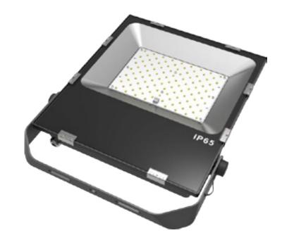
The Regus 100W is constructed from an aluminium moulding with the LED chips displayed in a standard array pattern. This creates optimum passive heatsinking as air travels over the fins on the heatsink.
